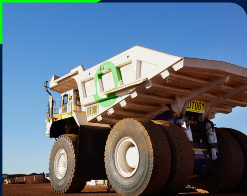
Fortescue's first prototype battery electric truck, Roadrunner, on site in the Pilbara
